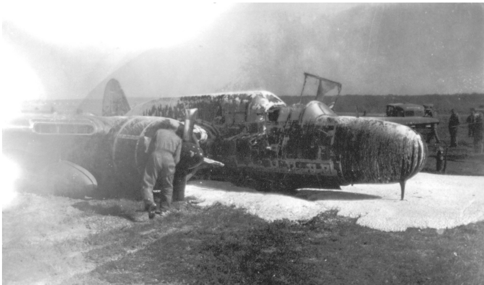
Lt. Bradford's P-61 at St. Dizier, France, April 9, 1945. Not enough lift on take-off when the gear was retracted resulted in grinding off the props. Note the installation of drop tanks, which were probably what caused the fire.
