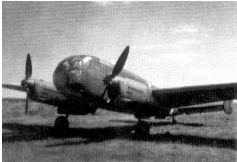
This is the German Seibel Si 204D liaison aircraft acquired by the 417th NFS after the war. The Squadron was getting quite a collection. This was a real performer, powered by two 600 hp Argus 411 engines, 364 kph.
