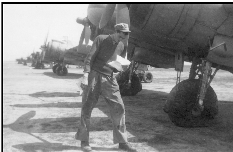
Bob Perry by row of Beaufighters, reading his mail. Note how the crews had to keep covers on the tires to prevent leaking engine oil from damaging them.
