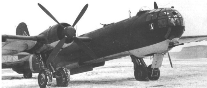
The Heinkel He 177 was the main German heavy bomber. Paired Daimler-Benz V-12 engines drove each propeller, so it performed as a 4-engine aircraft. Because the engines were "inverted" any leaking oil would cause fires on the hot exhaust manifolds.
