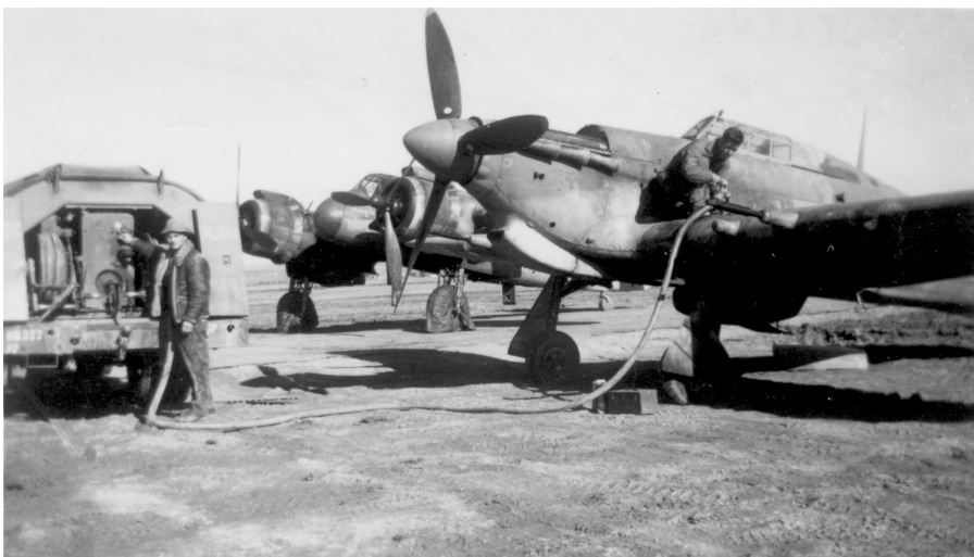
Hurricane LB595 was furnished to the 417th for pilot proficiency, which they seemed to relish. Here it is being fueled and prepared for its next outing. Note the aircraft was fitted with the tropical sand filter, required on single engine British aircraft operating in the desert. The Beaufighter was not so equipped and as a result dust and sand could quickly ruin an engine.
