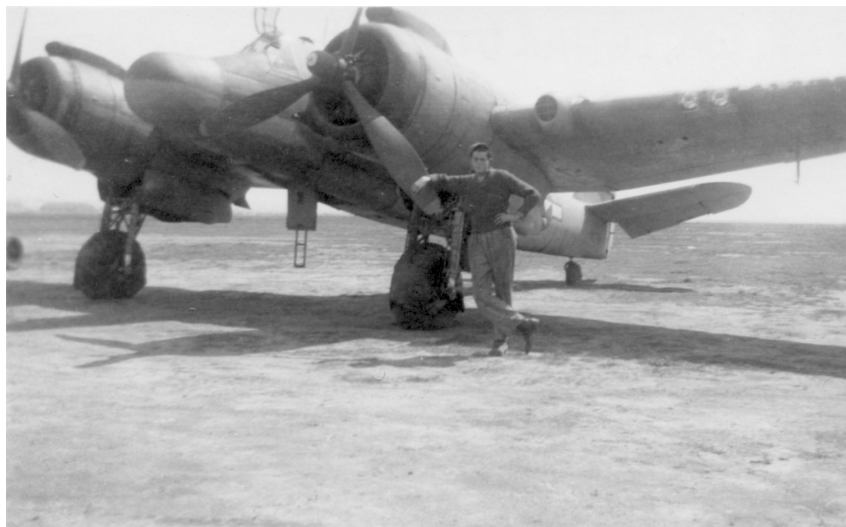
Hank Englehardt with one of the new Mk VIII (AI) equipped Beaufighter Mk VIs. Note the "thimble" radome on the nose and that all of the external antenna have been removed. The earlier Beaufighters were continually upgraded and repaired by the British and returned to operations. This is Beau V8875.
